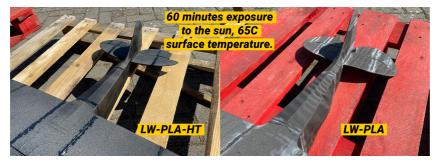
In comparison with the previous version of the filament, the new Light Weight PLA High-Temperature 3D print filament, made with Luminy® PLA, stood the heat without deformation by the sun.
