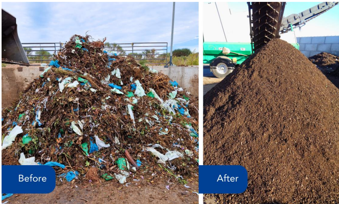
The start of the test (left): certified compostable shopping bags, trays, coffee capsules and films are mixed with organic waste at the. After composting ( on the right side) compostable plastics are disintegrated and
