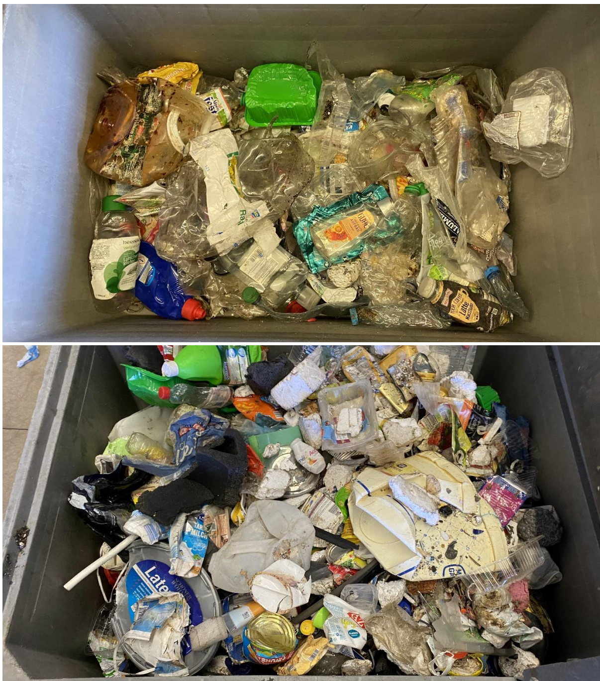
Figure 5: Test 2: Sorting fractions. Top: Ejected PET fraction. Bottom: Dropped others fraction.
