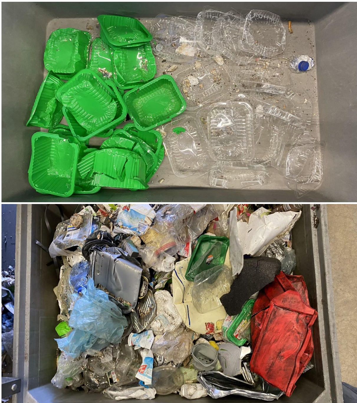
Figure 4: Test 1, Run 2: Sorting fractions. Top: Ejected PLA fraction. Bottom: Dropped others fraction.
