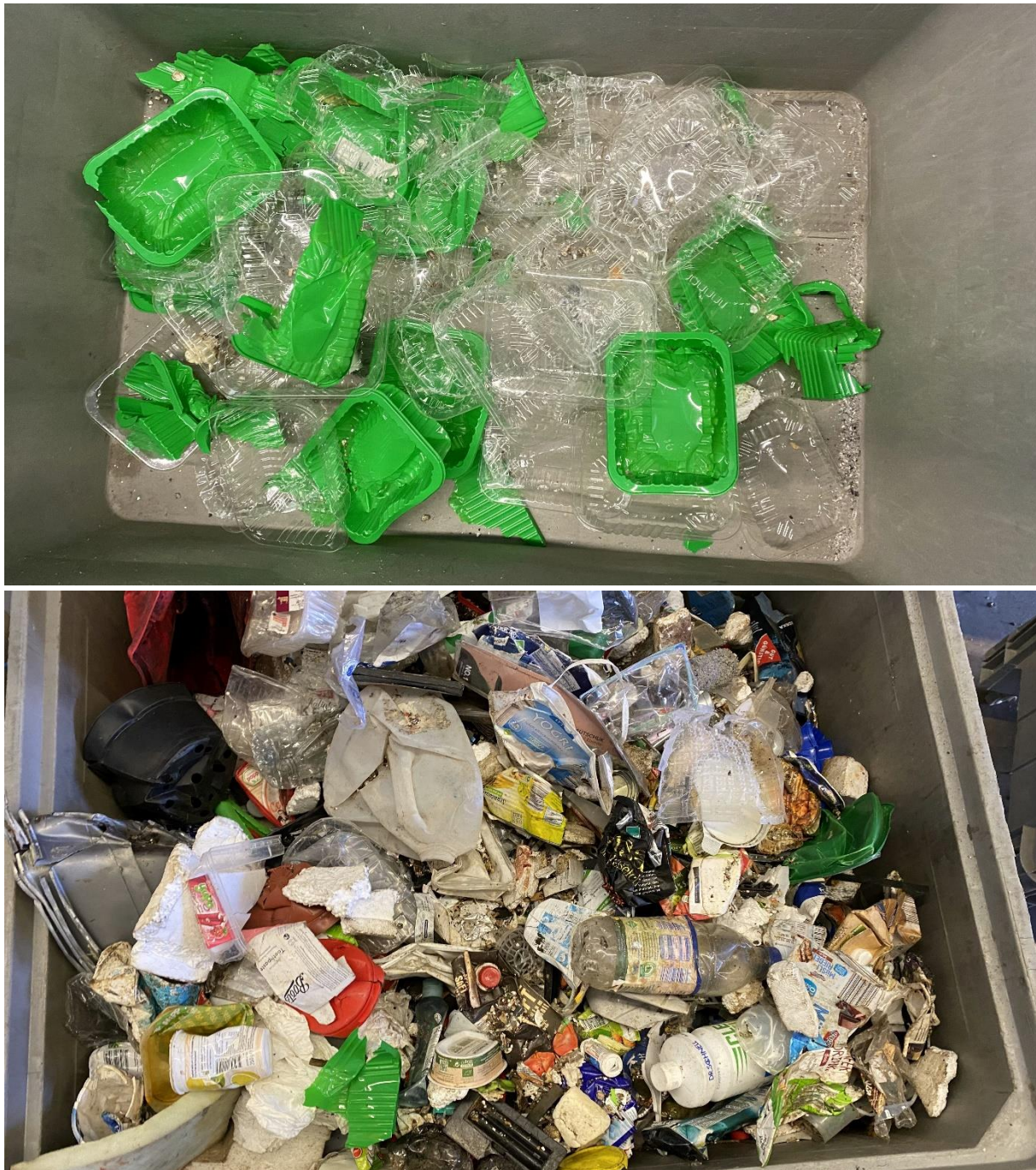
Figure 3: Test 1, Run 1: Sorting fractions. Top: Ejected PLA fraction. Bottom: Dropped others fraction.
